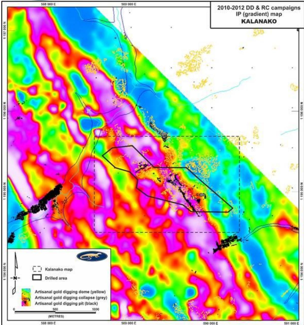
Figure 3 Induced Polarisation (IP) gradient map highlighting the structural location of the Kalanako prospect and the area drilled to date.
